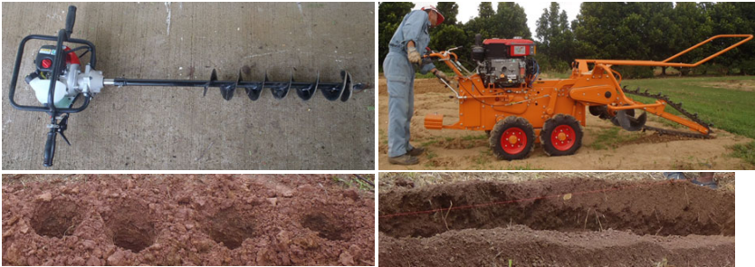
Fig. 1. Gas-powered portable auger (left) and self-propelled trencher (right) Left: Gas-powered portable auger (AGZ5010EZ, ZENNOH, Japan) attached with a drill (15 cm in diameter, 80 cm in length); Right: Self-propelled trencher (NF-827-II, KAWABE, Japan)
