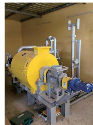
Fig. 3. External heating U-turn rotary kiln for calcination (Burkina Faso, INERA-Kamboinse)
