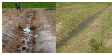
図2 植栽6ヶ月後の試験水路 Fig. 2. Test canal six months after installing (Left: Canal without vegetation, Right: Canal planted with ground covers)
