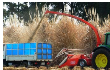
図3 「JEC1」の飼料作物収穫機「CHAMPION3000」による機械収穫効率 Fig. 3. Forage harvester (CHAMPION3000) showing the mechanical harvesting efficiency of JEC1
