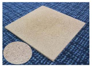
Fig. 1. Image of the binderless particleboard made from oil palm trunk (The magnified image of the surface is shown inside the circle.)
