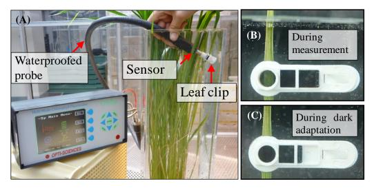
Fig.1. The measurement system of chlorophyll fluorescence in rice leaves underwater.
