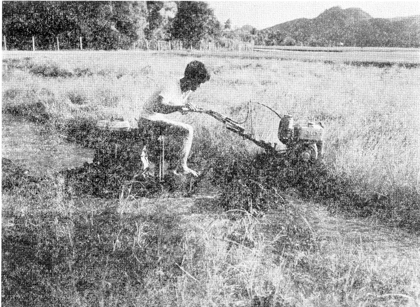
Fig. 9. Experimental four-wheel tiller in soft soil with deep hard pan.
