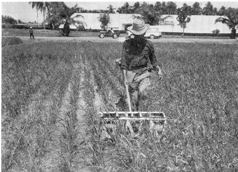
Fig. 5. Experimental three-row power weeder.
