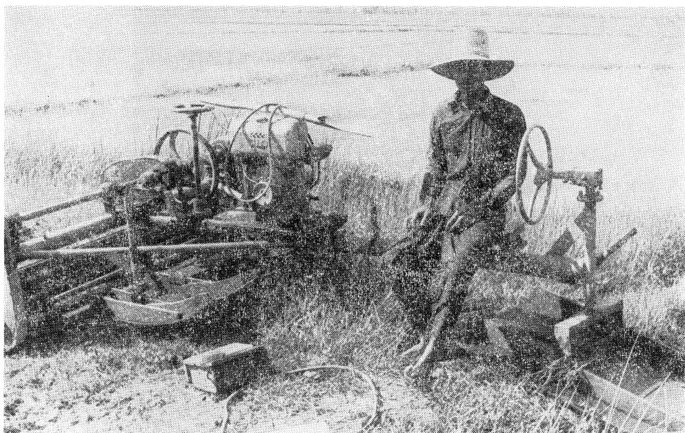
A hand-made puddling machine with depth and steering control units.
