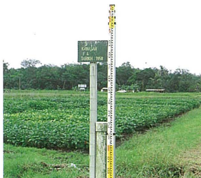
Annual surface subsidence of 3 cm has been observed since 1958 at Jalan Kebun (photo by S. Murayama)
