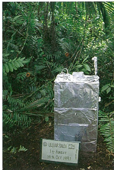
Measurement of \text{CO}_2 flux from peat soil surface (photo by S. Murayama)
