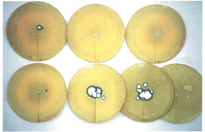
Honeydew spots on the bromocresol green-treated filter paper. When the honeydew drops on the filter paper, since blue spots appear, it can be distinguished from the plant sap (bottom, extreme right). The excretion of honeydew increases with the increase of the amount of sap that the BPH sucks from the rice plant. (Photo by K. Ito)
