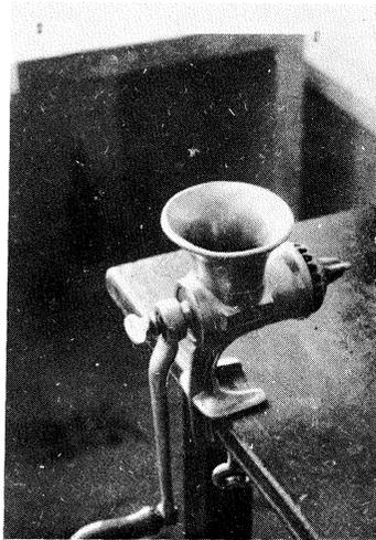
写真11. mincing machine (UPASI のTRS)
