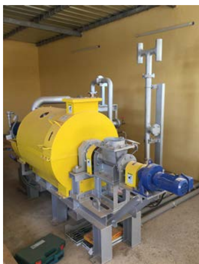
Fig. 3. External heating U-turn rotary kiln for calcination (Burkina Faso, INERA-Kamboise)
