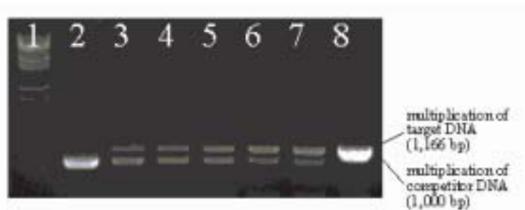
Fig. 1. An example of competitive PCR. Lane 1: DNA size markers ( \lambda - Eco T141 digest). Lane 2: Multiplication of competitor DNA. Lane 3-7: 1pM target DNA and competitor DNA, concentrations of each lane are 100pM, 10pM, 1pM, 100nM, and 10nM, respectively. Lane 8: Multiplication of target DNA.
