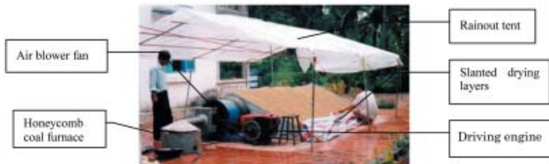
Fig. 1. Unfulled rice dryer.
