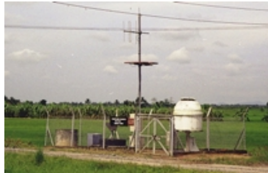
Photo 2. Rainfall station equipped with a VHF radio.
