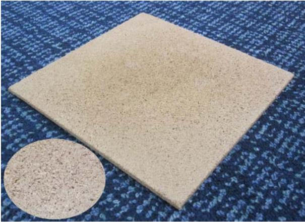
Fig. 1. Image of the binderless particleboard made from oil palm trunk
