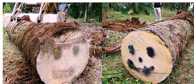
Fig. 6. Spray tests using iodine solution to determine sugar-accumulating old oil palm trunks (OPT). Left: non-accumulating OPT; Right: sugar-accumulating OPT
