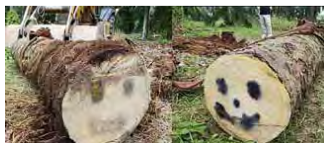
Fig. 6. Spray tests using iodine solution to determine sugar-accumulating old oil palm trunks (OPT). Left: non-accumulating OPT; Right: sugar-accumulating OPT
