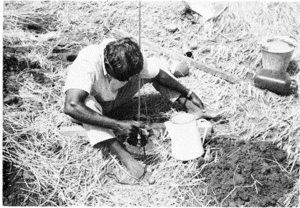
Photo.8 Permeability test by dry auger hole method in the detailed study lot during non-irrigation period.
