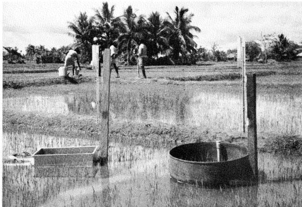
Photo.5 Lysimeter for the measurement of evapotranspiration (right) and N-type water requirement measuring apparatus (left)
