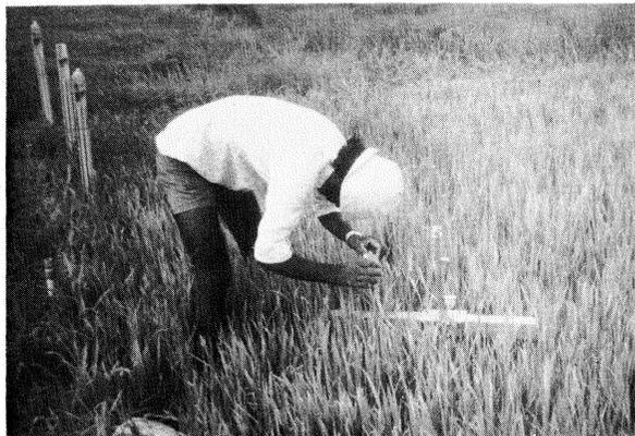
Photo.9 Permeability test by tube method in the detailed study lot during irrigation period.
