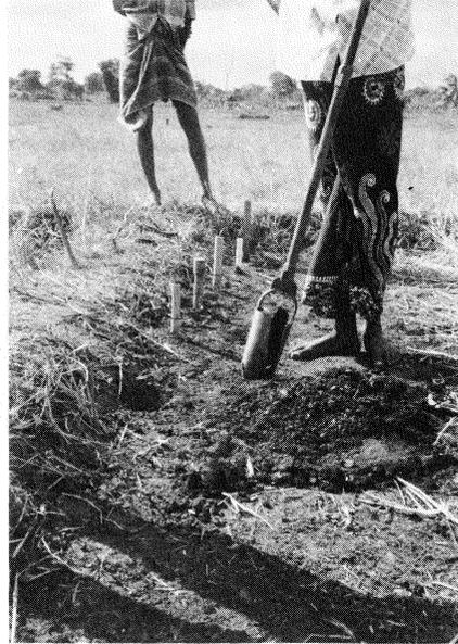
Photo.12 Installation of pipes for measuring hydrostatic pressure head in the detailed study lot.
