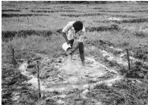
Photo.23 Preparation of a test plot for percolation control method (bentonite dressing (mixing))
