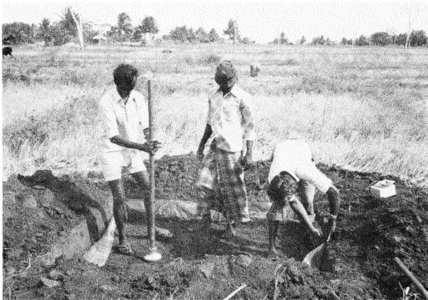
Photo.19 Preparation of a test plot for percolation control
