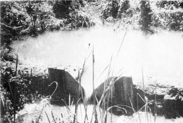
Photo.16 Water balance study in paddy fields extending over a small area (9.7ha) (measurement of discharge by 90° V-notch weir in drainage)
