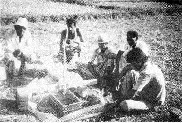
Photo.15 Measurement of seepage and percolation through plowsole in the detailed study lot.
