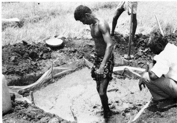
Photo.20 Preparation of a test plot for percolation control
