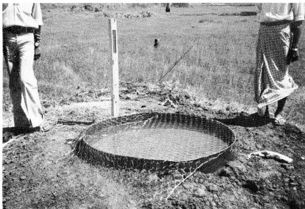
Photo.6 Pan evaporation of special installation ( $\phi 120\text{cm}$ )
