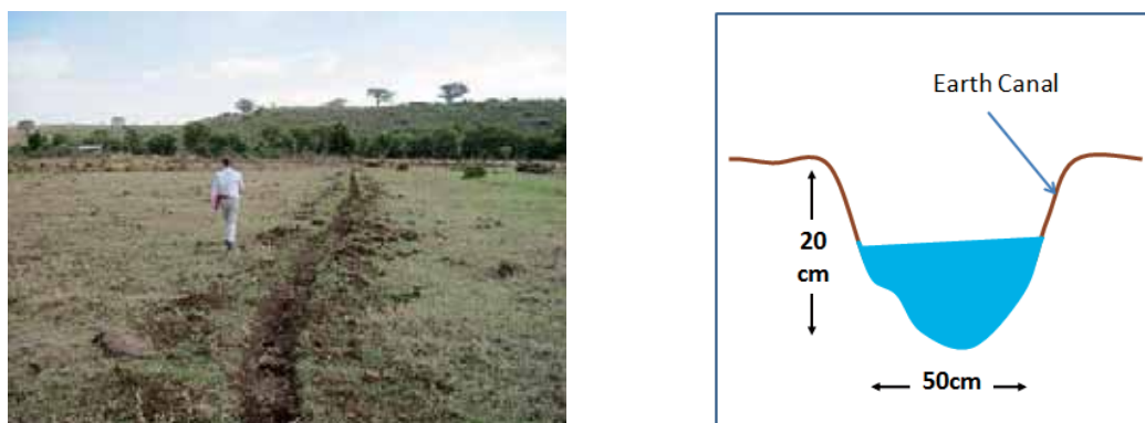
Figure 4-6 Earth canal (a) and Cross Section (b)
