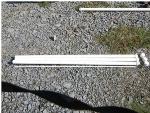
Reference Photo 1. Groundwater level measurement pipes
