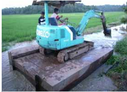
Pic.6.10 Dredging shovels floating on barges in canal
