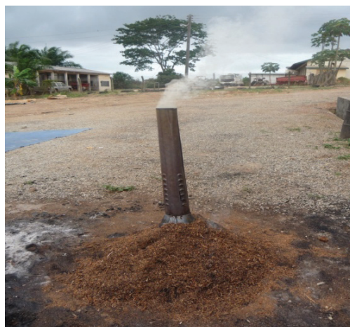
Charring process is going on for 1 to 2 hours
