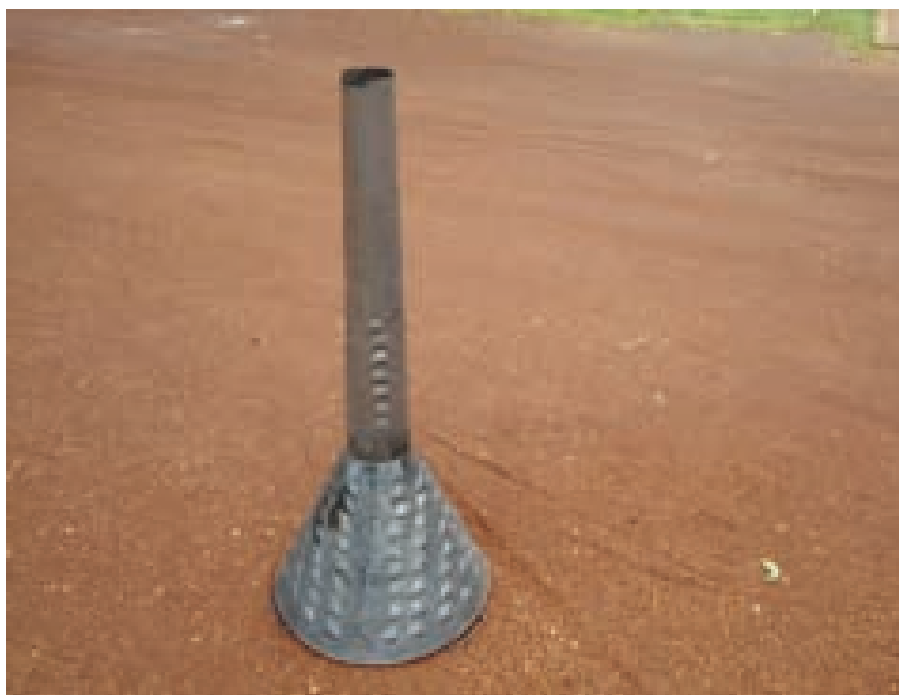
Plate 1-4-1: A Ghanaian-made complete replica of the Kuntan-charring apparatus commonly used in Japan.
