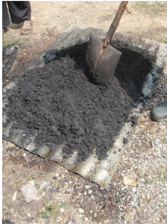
Plate 4-3-6: Resulted P-enriched biochar made from sawdust.
