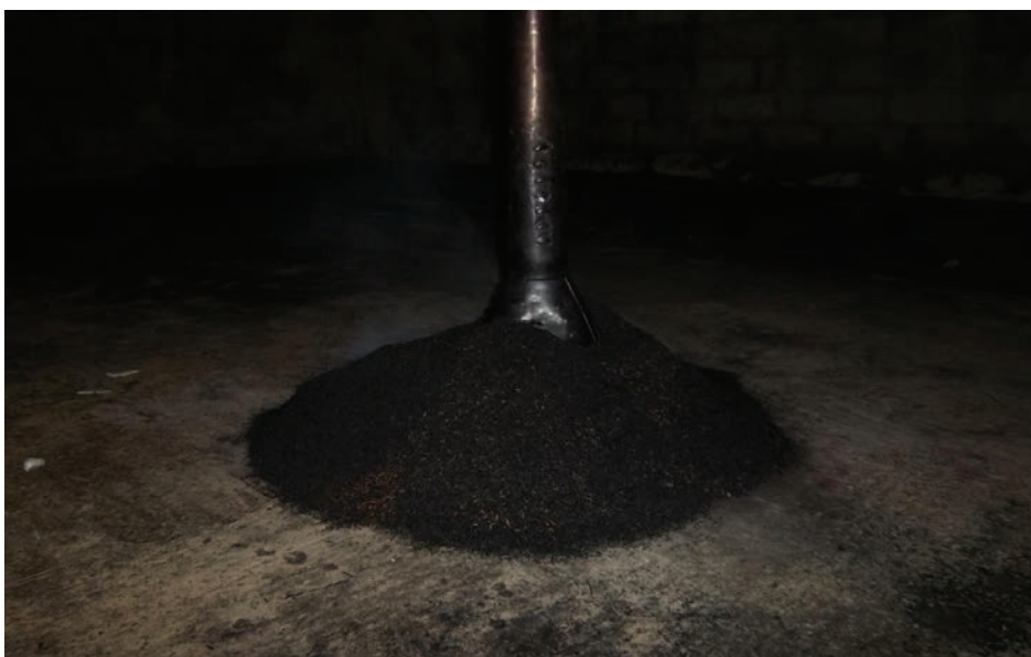
Plate 1-4-9: Charring process completed all the material turns black.
