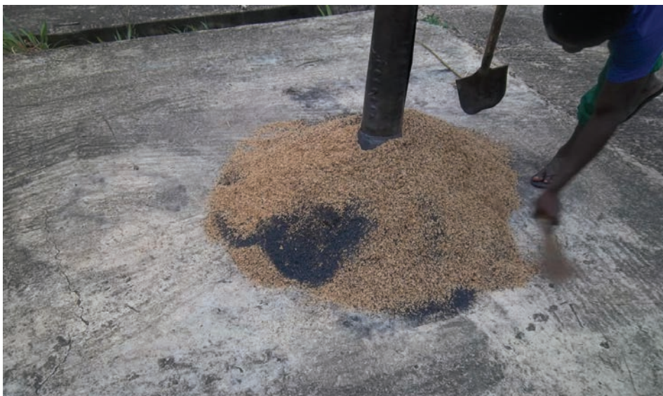
Plate 1-4-8: Turning of charring material.
