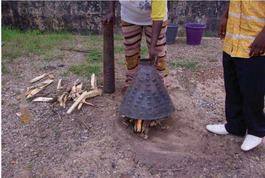
Plate 4-3-2: Fire is covered by a charring apparatus.
