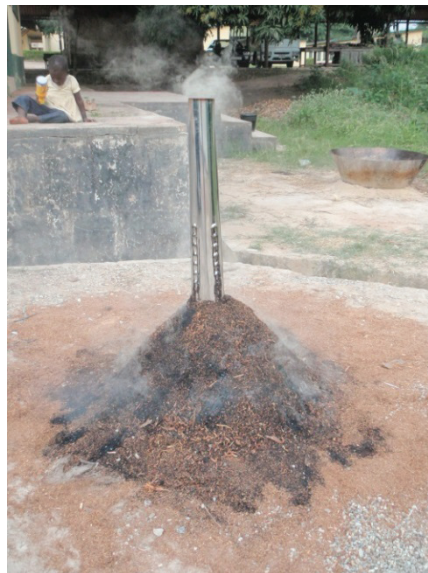
Plate 4-3-5: Charring process is going well with increasing of black parts in sawdust.
