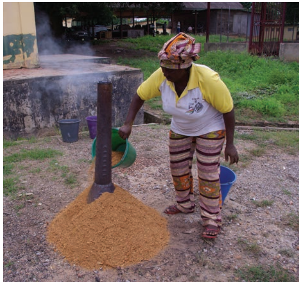
Plate 4-3-3: Pouring the mixture of PRs and sawdust.
