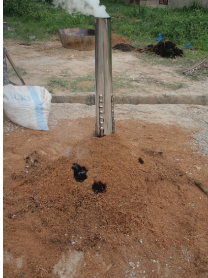
Plate 4-3-4: Black spots appeared on the surface of the heap.
