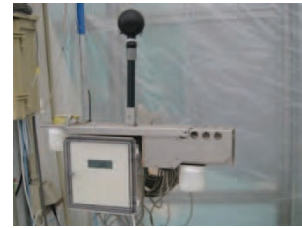
Figure 1 Wet-bulb globe temperature (WBGT) sensor , which is compliant to UECS and can be used for labor management.
