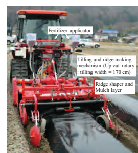
Figure 1 Simultaneous tilling, ridge-making, and mulch-laying machine and the arrangement of its blades
