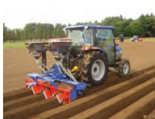
An in-ridge partial fertilizer application machine
