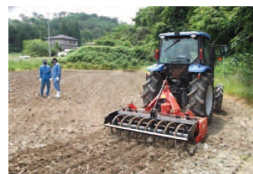
Surface soil crushing by a tractor equipped with a power harrow
