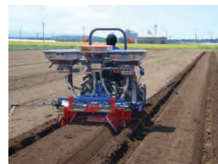
An in-low-ridge partial fertilizer application machine
