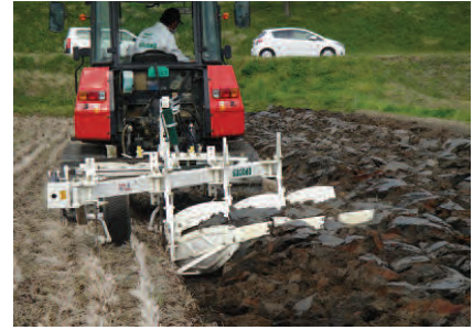
Soil turning in a paddy field by a plow with jointers
