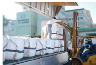
Loading of round bales of fermented TMR using a round bale handling assister
