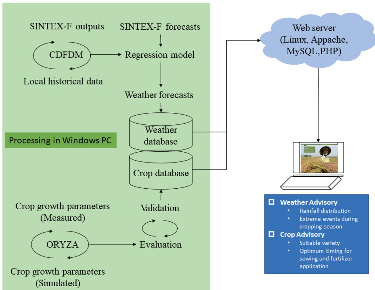
**Fig 1. Conceptual flow of database development for WeRise** (Any version of windows is accessible, and no macro is used for operation of WeRise)
