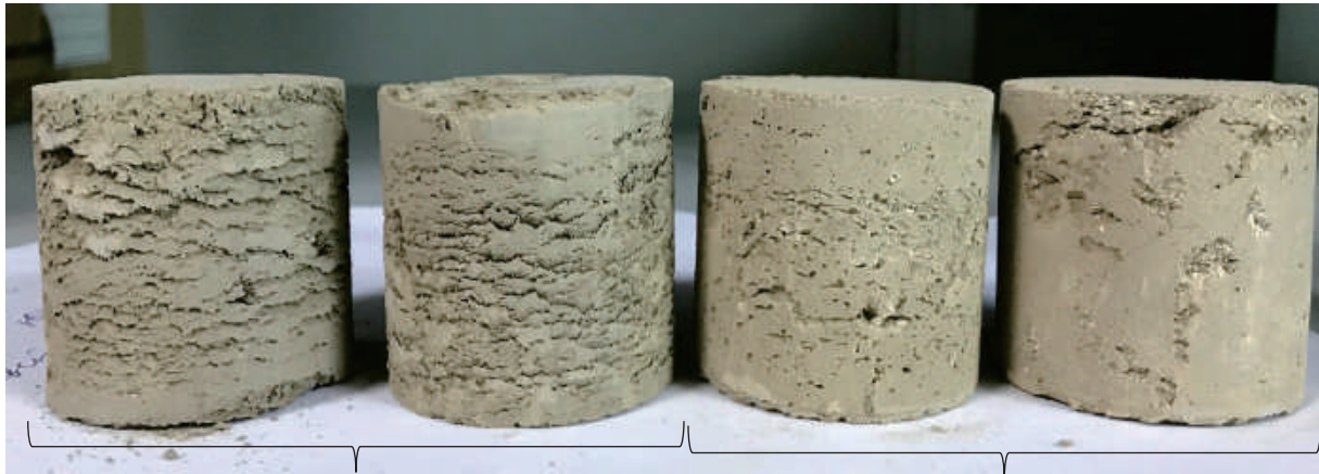
15 cm in depth Left: 30 cm in depth, right 60 cm in depth Fig. 8 Soil samples after leaching experiment (disturbed hardpan, after drying)
