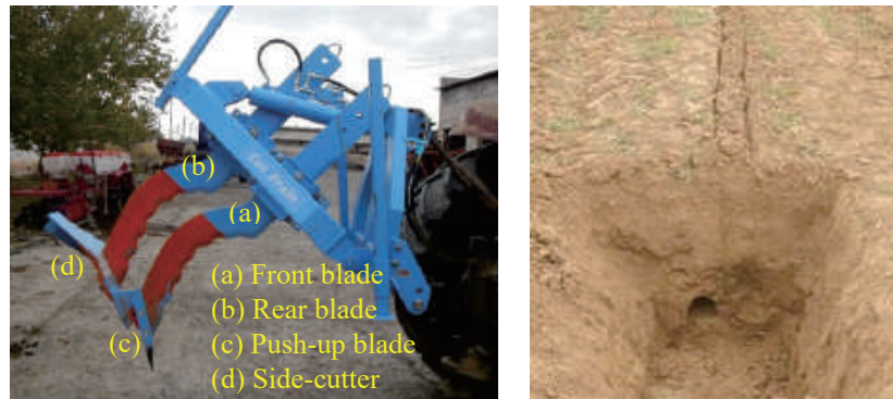
Fig. 1 Drain-drilling machine and cavity of Cut-drain
