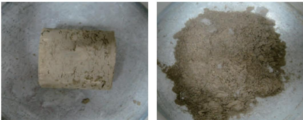
Fig. 7 Slaking test. Left, before flooding and right, after 5 minutes
