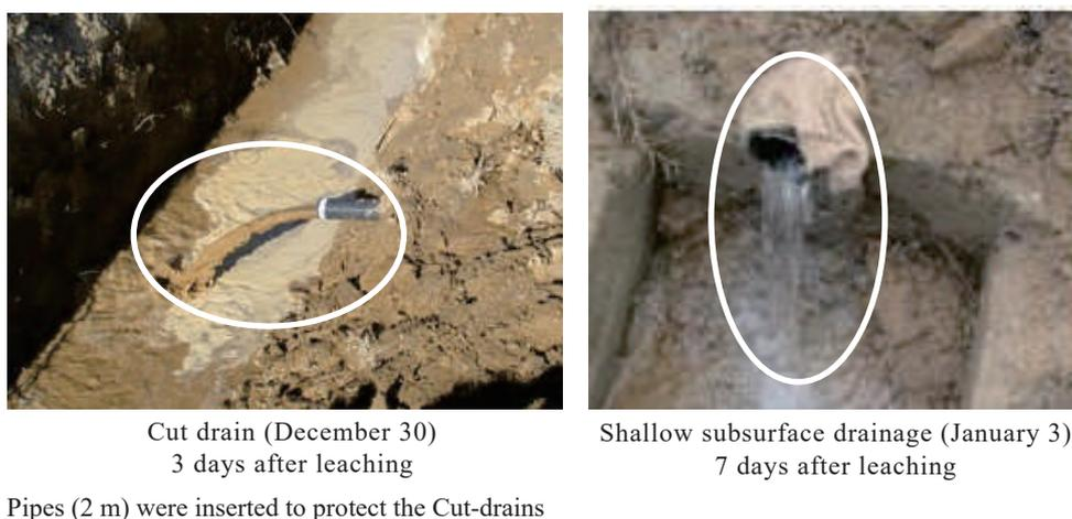
**Fig. 7** State of discharging from outlets after leaching
