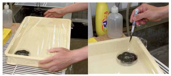
Fig.18. Make the holes for the exchange the air in rapped box
