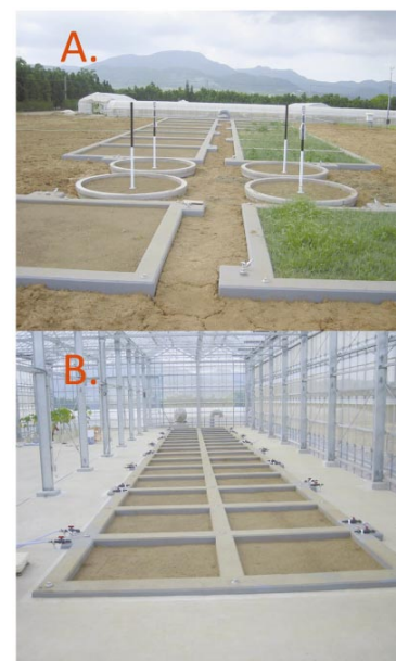
Fig. 2. Experimental setup A. Lysimeters and weighing lysimeters in the field (outdoors) B. Lysimeters in the greenhouse (indoors)
