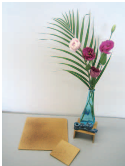
Fig. 3. Binderless particle board produced from oil palm trunk
