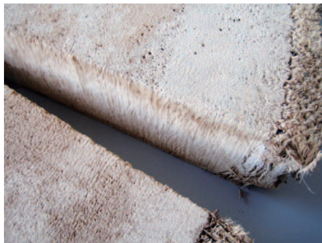
Fig. 2. Cross-section of oil palm trunk after drying (Note: While standing, it may look like a “tree”. However, the vascular bundles that appear in the cross-section are scattered and there are no cambium and no secondary growth.)
