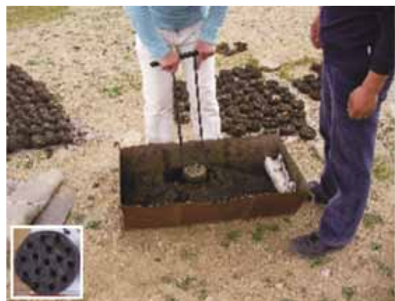
Manufacturing fuel blocks (Bottom left picture: a fuel block) (Photo by: K. Kimura)
