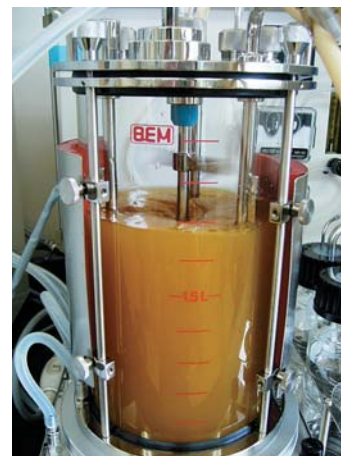
Fermentation test using the sap from an oil palm trunk
