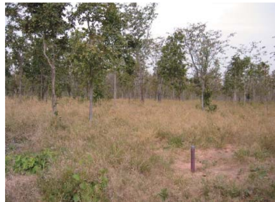
Photo 1. Top of the hill - Land use is forestry. Groundwater level was 12.23 m deep (depth of the well is 30 m) as measured on December 21, 2005.
