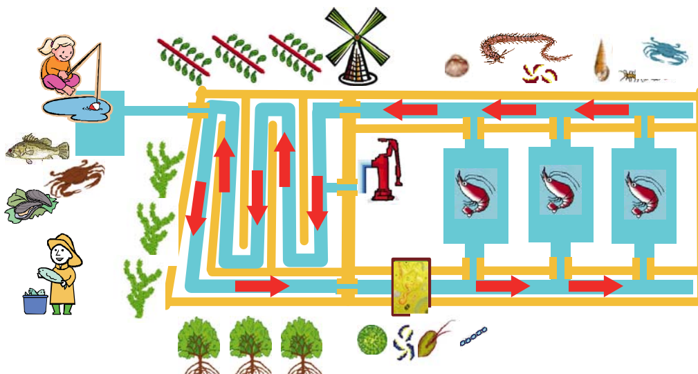
Fig. 1. Environment-friendly, recycling-oriented prawn aquaculture system utilizing the natural ecological functions of benthic and planktonic organisms, mangrove stands and seaweeds
