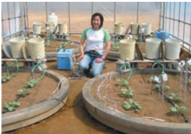
Photo 2. Measurement of water use in plants using weighing lysimeters
