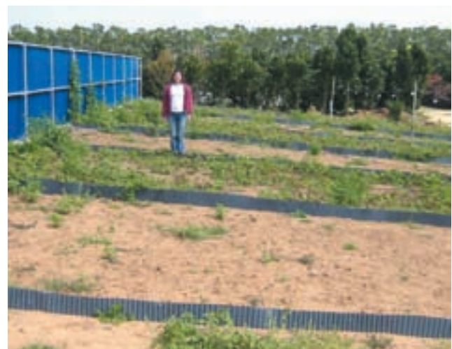
Photo 3. Analysis of soil erosion using artificially-developed slopes
