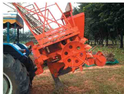
Fig. 2. A newly developed sugarcane planter with subsoiling chisel.
