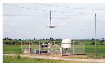
Rainfall station with VHF radio
