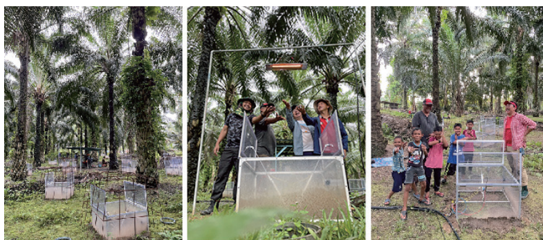
Photo 2. Automatic multi-channel chamber system installed in an oil palm plantation in Malaysia with the cooperation of the National Institute for Environmental Studies. Warming experiments that simulate future climate change are also conducted (center).
