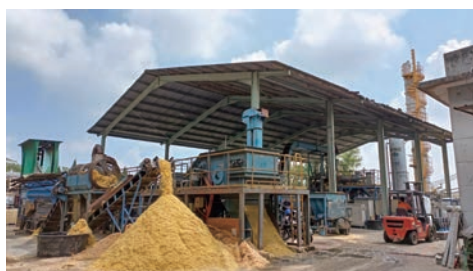
Photo 1. Demonstration site of the Multi-Biomass Treatment Process under the SATREPS project. This facility served as a hub for developing technology to convert diverse biomass into high-quality pellets, which were supplied to research institutes and companies in both Japan and Malaysia for application studies.
