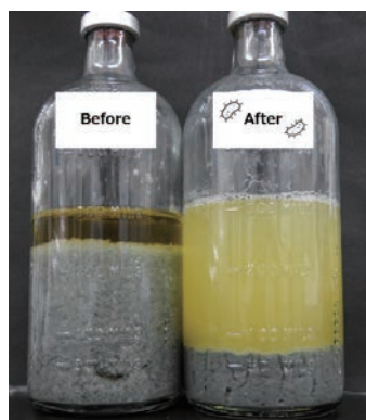
Photo 1. Microbial saccharification using untreated waste magazines. The microbes' own enzyme systems break down biomass, and the saccharified liquid can be directly used for methane fermentation.
