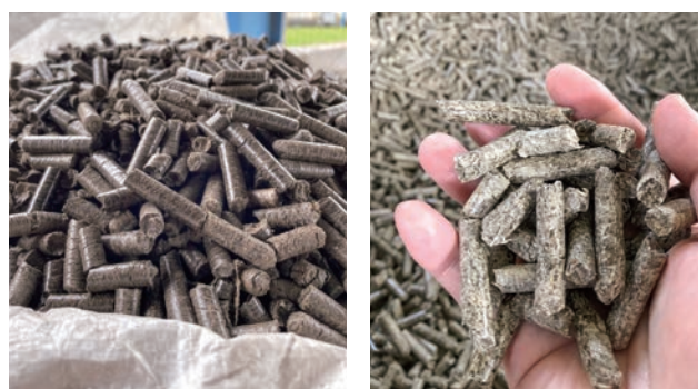
Photo 2. Biomass pellets produced from empty fruit bunches (EFB) and oil palm trunks (OPT)
