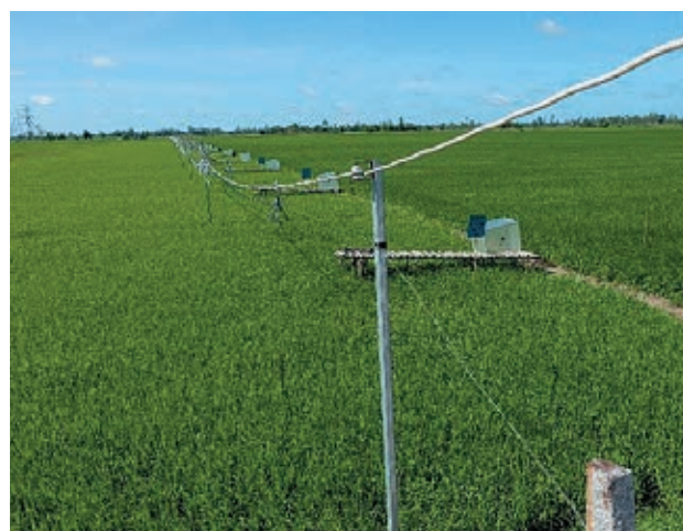
Photo 2. Measurement of GHG emissions from paddy fields in Mekong Delta, Vietnam. The alternate wetting and drying (AWD) technology for reducing GHGs contributes to SDG 13 (Climate Action).
