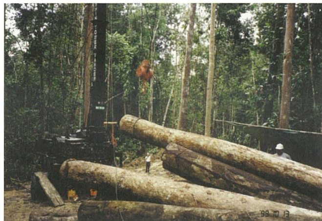
A trial operation of the cable logging system
