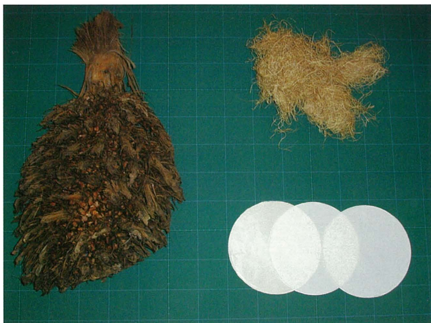
Empty fruit bunch (left), fibrous strands of EFB (right top) and paper sheets made of TCF-bleached EFB pulp (right bottom).
