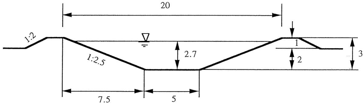
Fig. 2. Standard cross-section of proposed small pond
