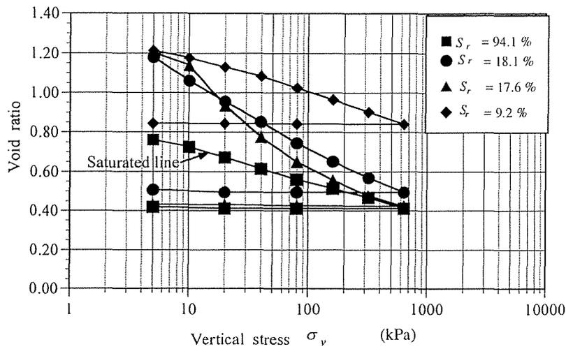
Fig. 4. Relationship between void ratio and vertical stress of Yellow soil obtained from oedometer tests<sup>4)</sup>
