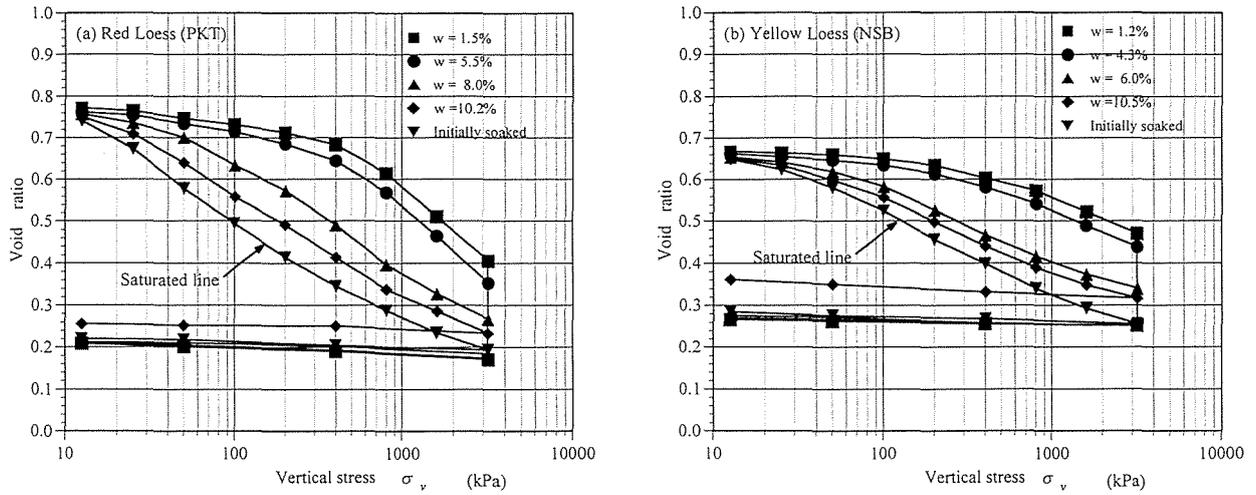
Fig. 3. Oedometer test results of undisturbed Red and Yellow Loesses (data from Udomchoke<sup>8)</sup>)
