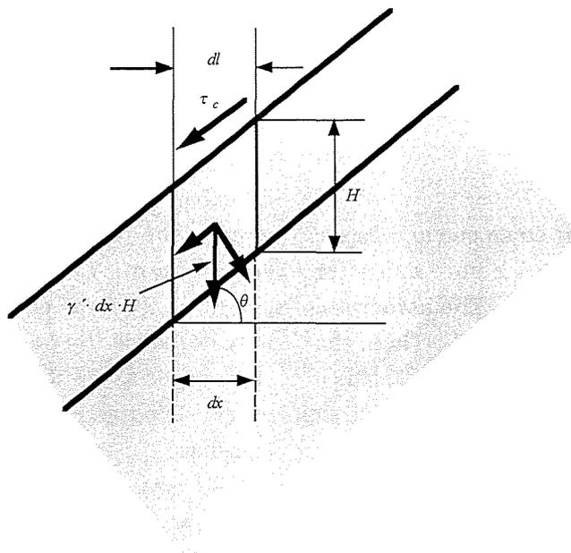
Fig. 6. Slope resistance to sheet erosion
