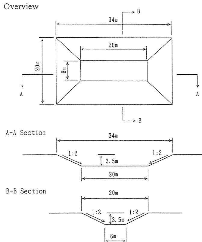
Fig. 1. Standard small farm pond recommended by DLD<sup>2)</sup>
