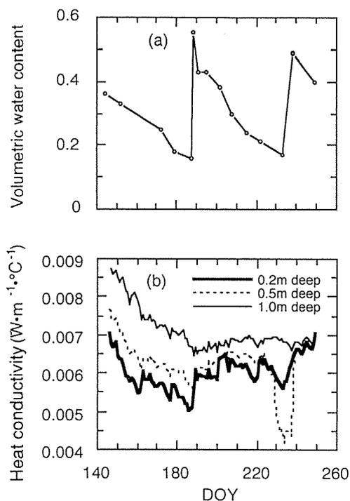
Fig. 8. Changes in volumetric soil water content and heat conductivity (1995)
