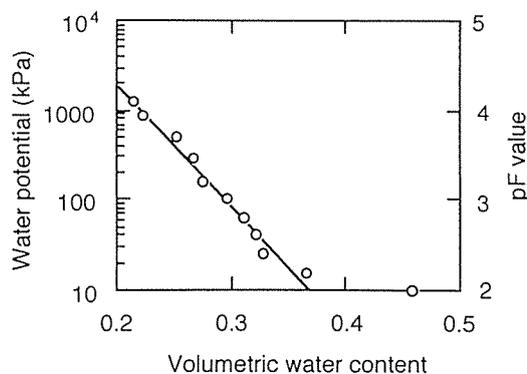
Fig. 9. Relationship between volumetric water content and water potential of the soil
