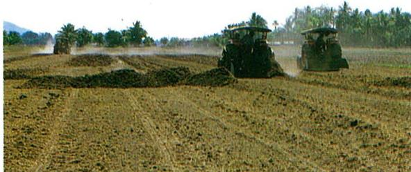
Plate 1. Land levelling by tractor with rear bucket
