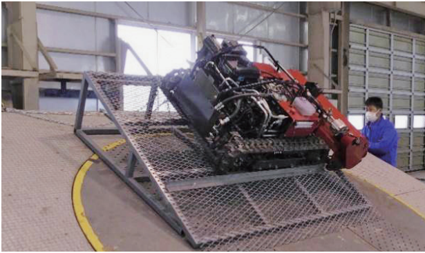
Fig. 4. Measurement of static tipping angle
