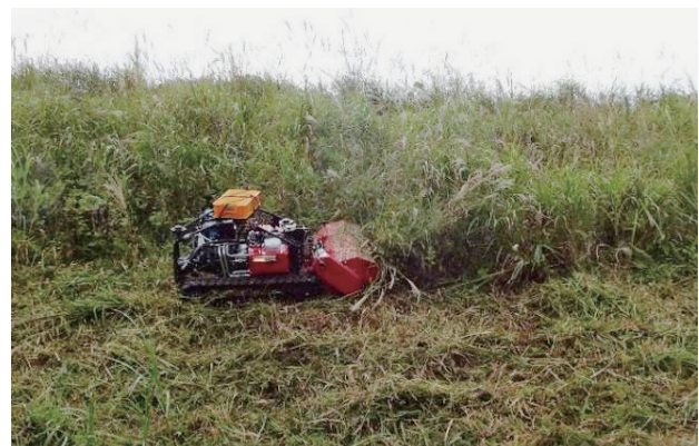
Fig. 6. Mowing on a steep slope (max. 39°)
