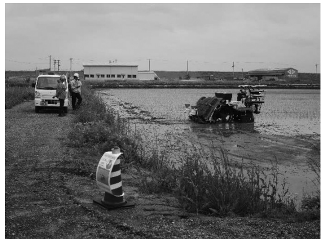
Fig. 4. A robot rice transplanter doing farm work
