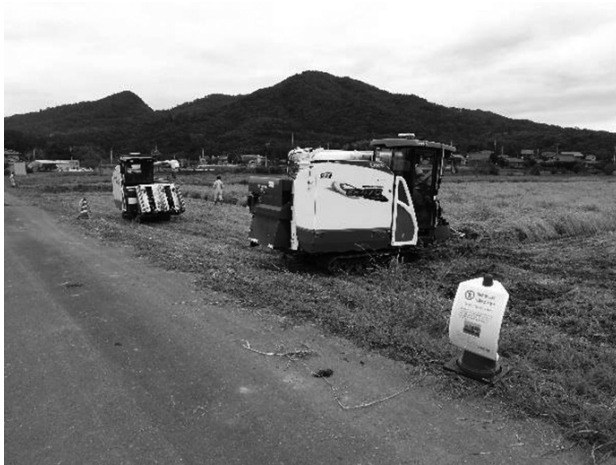
Fig. 5. A robot combine harvester doing farm work
