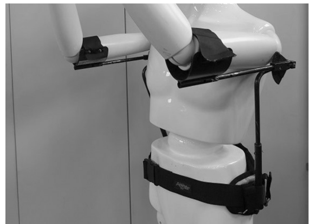
Fig. 1. Overview of the arm-raising work assistance tool
