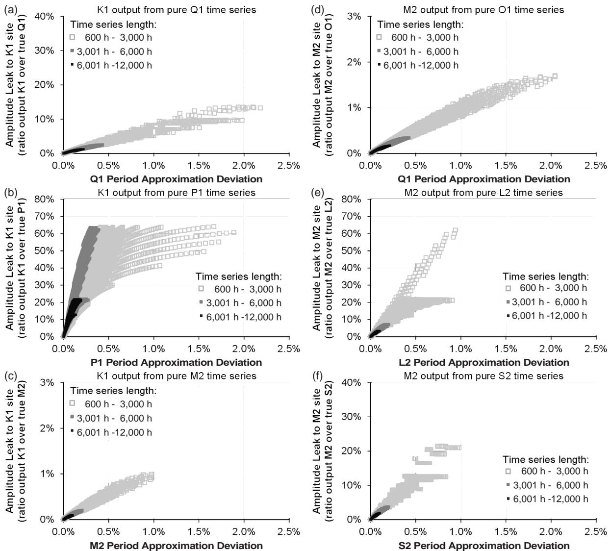
**Fig. 7. Amplitude leakages for six combinations of the tidal constituent contained in the analyzed time series and the tidal constituent frequency site affected by the leakage, plotted against the PAD of the contained constituent**
