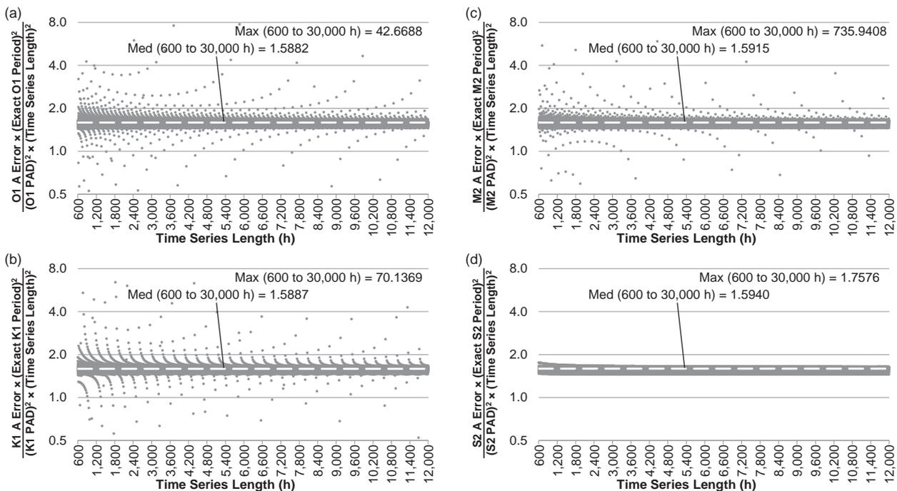
**Fig. 5.** Values calculated using Eq. (4) or (5) plotted against the analyzed time series length for the (a) O1, (b) K1, (c) M2, and (d) S2 constituents
