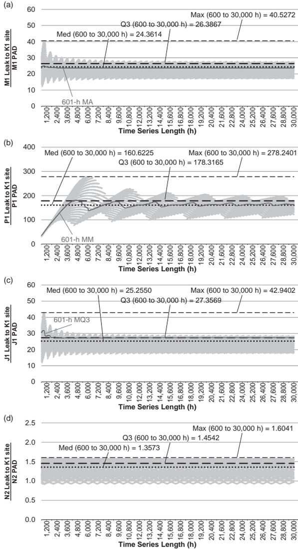
**Fig. 8. Ratios of output amplitude leakage over the PAD of the tidal constituent contained in the time series plotted against the analyzed time series length, for leakages of (a) M1 constituent to K1 site, (b) P1 to K1, (c) J1 to K1, and (d) N2 to K1**
