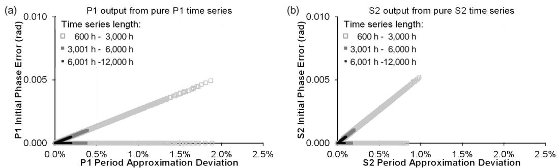
**Fig. 6. Output initial-phase error magnitudes of the (a) P1 and (b) S2 constituents, plotted against the period approximation deviation of the constituent**
