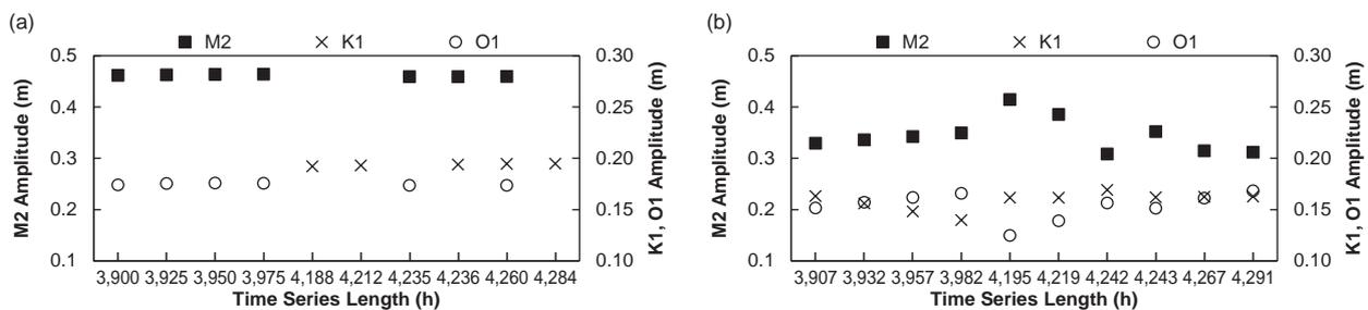
**Fig. 10. Amplitudes output from real groundwater-level observation time series data by Fourier analysis (a) with time series lengths selected by the current derived criteria and (b) with unselected lengths**
