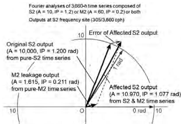
**Fig. 3. Polar plot showing three Fourier analysis outputs at the S2 frequency site**
