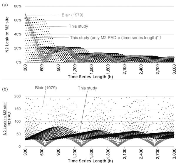
**Fig. 9. Comparison between the results of Blair’s (1979) error prediction formula and the Fourier analysis of this study**
