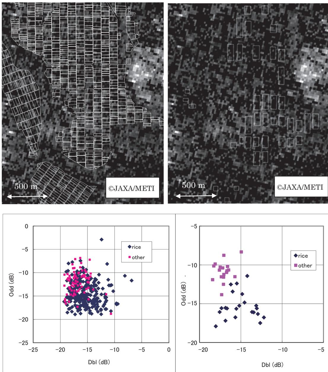
Fig. 9. Odd scatter component image of 24<sup>th</sup> August 2008 and scatter plot (left side: parcel scale, right side: block scale)
